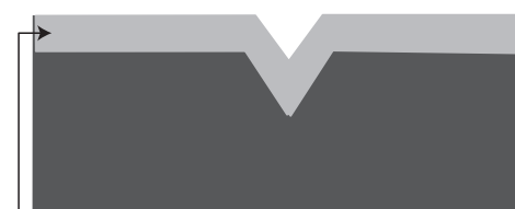
Figure 3 The protective coating is quickly restored through the rapid self-repairing quality of the chromium rich film.
